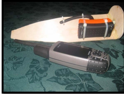
GPS Tracker on nose cone insert with hand-held GPS receiver
