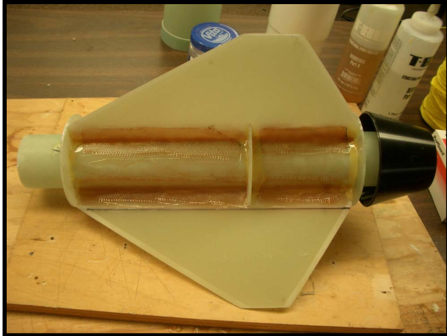
Fin-to-Motor Tube Mounting
