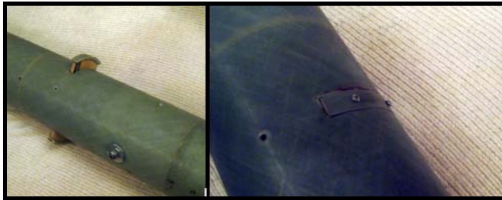
Air brakes extended
