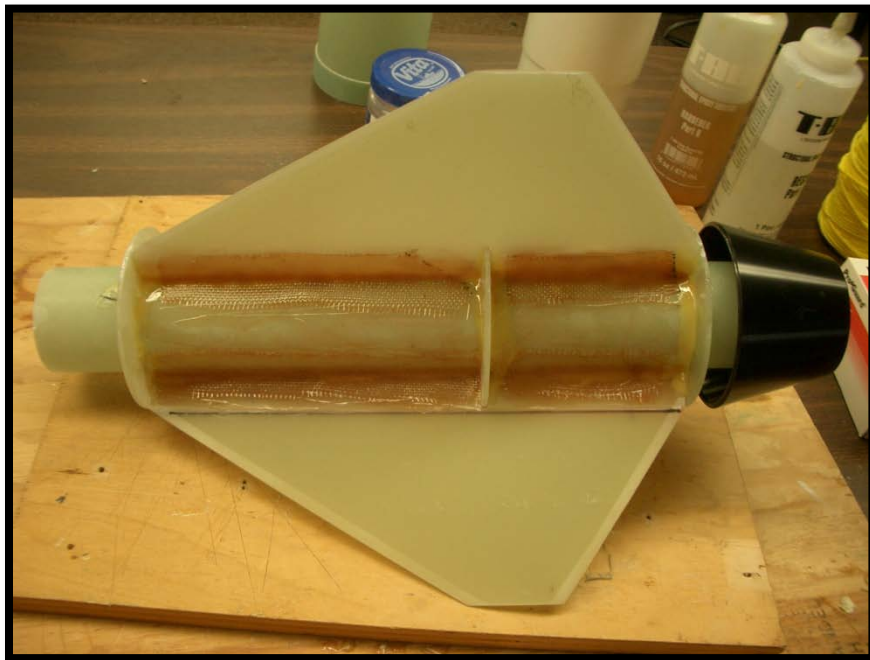
Figure 21 - Fin-to-Motor Tube Mounting
