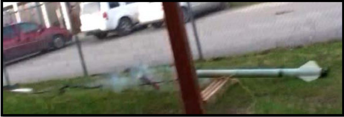
Figure 5 - Drogue Ejection Ground Test
