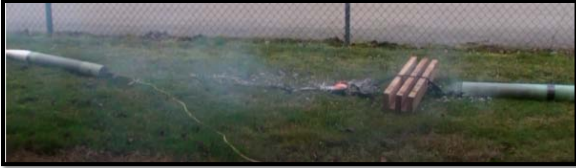
Figure 6 - Main Ejection Ground Test
