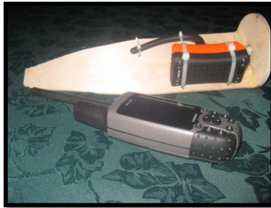
Figure 17 - GPS Tracker on nose cone insert with hand-held GPS receiver
