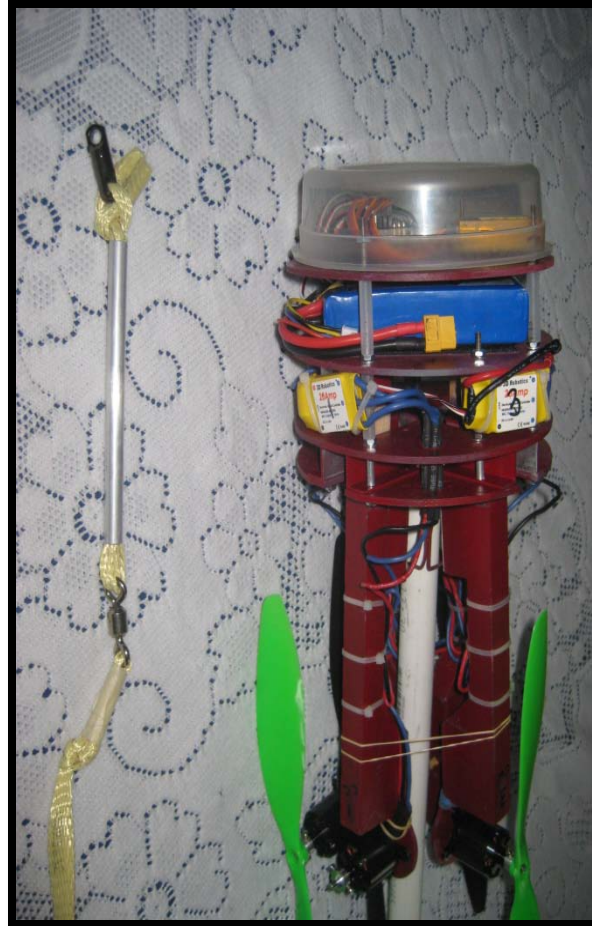
Tow Harness, Aluminum Pass Through, Pedestal and Protective Cap on MV Mini-Mincer
