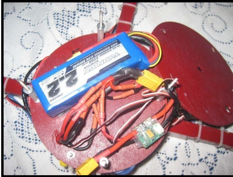
Deck 3 with Battery and Power Distribution Unit
