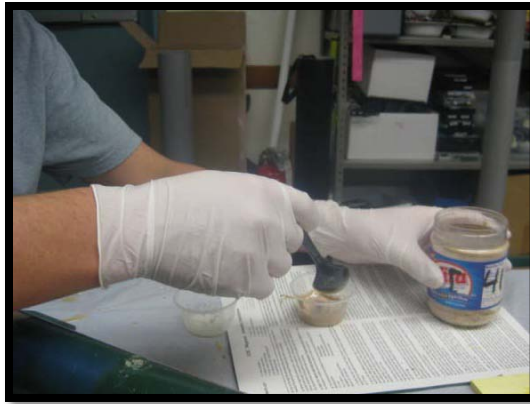
Figure 34, PPE latex gloves while working with epoxy resin
