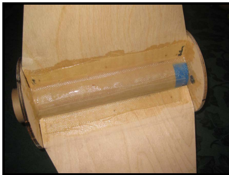
Figure 5 – Through-the-Wall Fin Attachment
