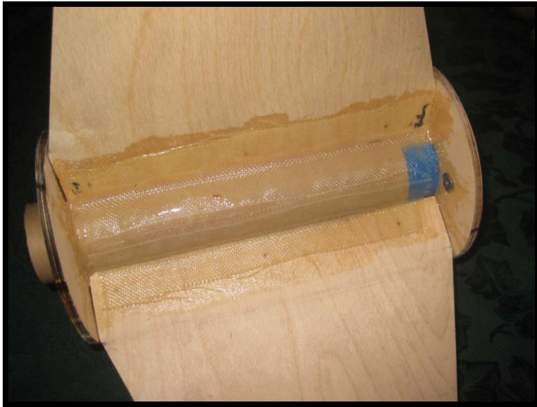
Figure 17 – Fin Can Illustrating Fiberglass Reinforcement
