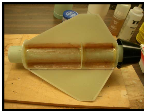
Figure 6, Typical Through the Wall Fin Attachment
