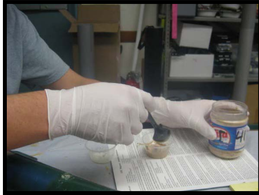
Figure 29, PPE latex gloves while working with epoxy resin
