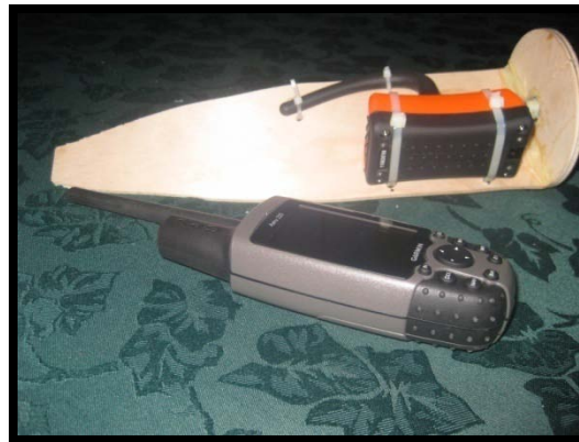
Figure 3, GPS Tracker on nose cone insert with hand-held GPS receiver
